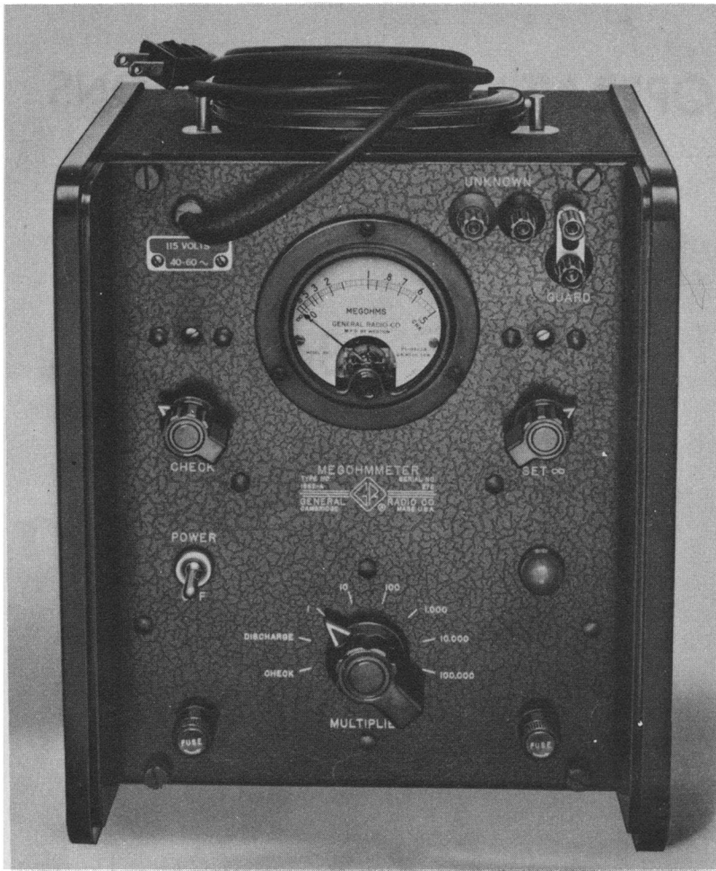
Panel View of the Type 1862-A Megohmmeter
